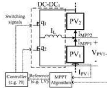
Fig. 2 Maximum power point tracking combined with regional data.
